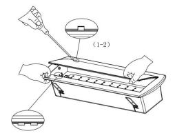
2. Open the LED board with a screwdriver.
