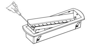
3. Connect the device to power supply.
