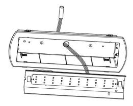
4. Put the fixture into the wall and fix with the spring.
