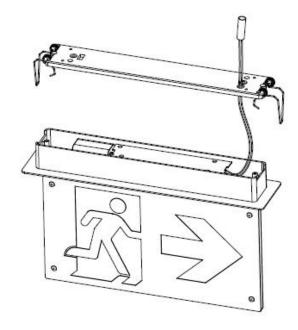
3. Recess the fixture to the ceiling through the spring.
