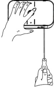
2. Knockout in back of mounting plate and push wires through the hole.
