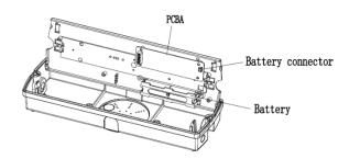
5.Push the fixture back and twist on the screws. Restore power and cut off again, the LED will work with backup battery on emergency mode. Restore power again to complete the installation.
