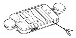
2. Knockout in back of mounting plate and push wires through the hole.
