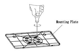
3. Securely attach mounting plate to J-box (not provided).
