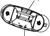
Battery connector 6. Snap fixture onto mounting plate and ensure no wires are pinched. Make sure unit is fully attached.
