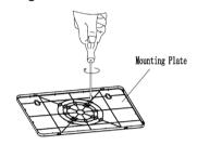
Securely attach mounting plate to J-box (not provided).
