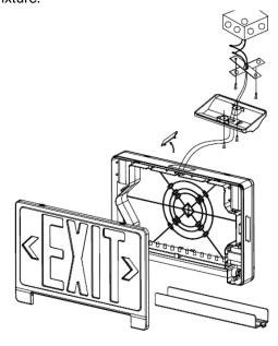
2. Reference step 3 – 6 in wall mounting above for ceiling mounting.
