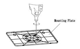
3. Securely attach mounting plate to J-box (not provided).
