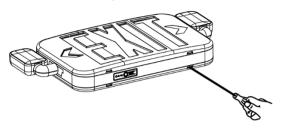
2. Knockout in back of mounting plate and push wires through the hole.
