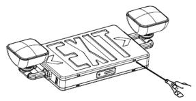
2.Knockout in back of mounting plate and push wires through the hole.
