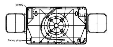
5.Snap fixture onto mounting plate and ensure no wires are pinched. Make sure unit is fully attached.
