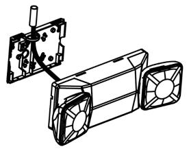
3. Reference step 4 - 7 in wall mounting above for ceiling mounting.
