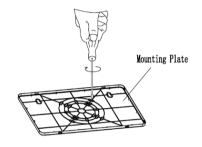
3. Securely attach mounting plate to J-box (not provided).
